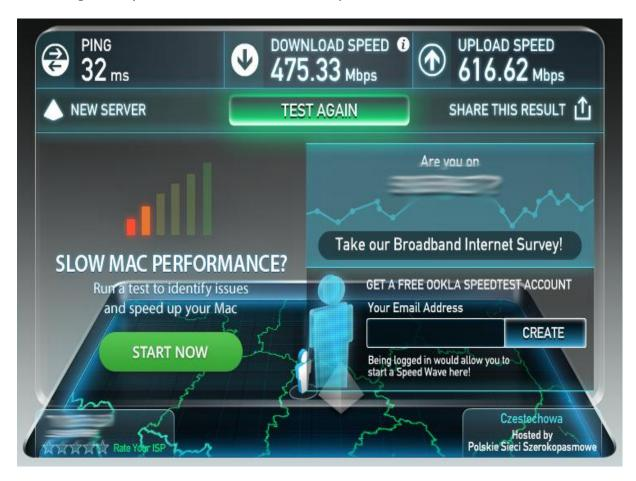
The results are very satisfying. Achieved download speed is 500 Mbit/s with 600 Mbit/s of upload. Nowadays, this is a very good result. Any inaccuracy in the measurement of bandwidth and undervaluation of download/upload speed may result from the current server load, on which the measurements were made.
