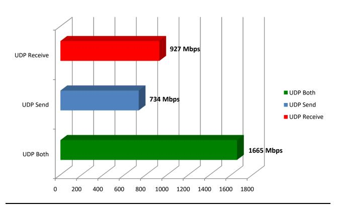
In the above chart **EXTRALINK TITANIUM GPON / 4GE / POTS / WIFI** stands for its great throughput performance. Virtually, one of four Gigabit Ethernet ports has been used 100%. This is very good achievement because the test has been carried out during rush-hour in the network.
