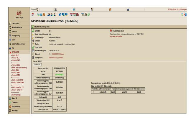
After you add the device, LMS system by using SNMP protocol enables you to get access to detailed information related to the connection parameters such
